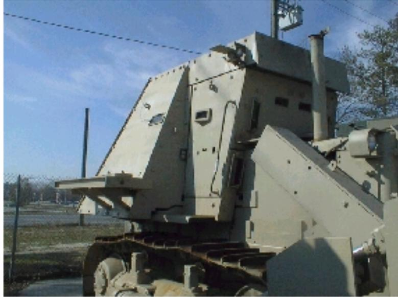
Figure D-5. Tractor Protective Kit
