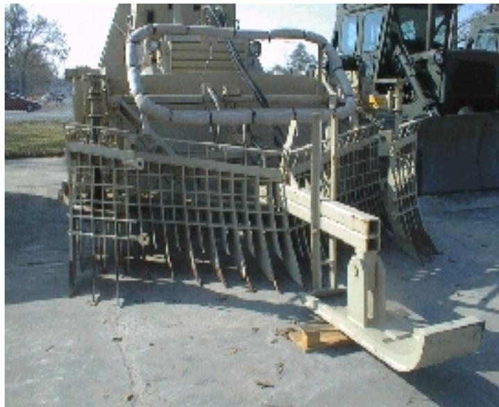
Figure D-6. Full Width Mine Rake mounted on D7 dozer.
