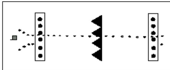
**Figure 6-06. Marking a complex obstacle as a system.**
